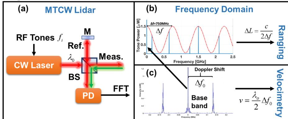
Fig. 1 (a) MTCW Lidar configuration, (b) ranging and (c) velocimetry data extraction in frequency domain.
