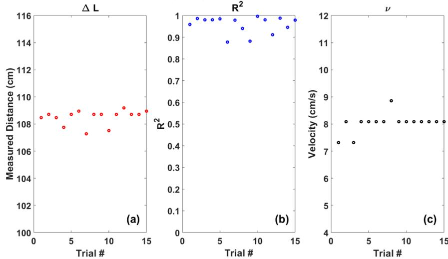
Fig. 2 Simultaneous ranging and velocimetry results for 15 trials while the target is moving with  $v = 8$  cm/s. (a) Ranging, (b) corresponding  $R^2$  of the sine fitting, and (c) the measured velocity at the corresponding instance.
